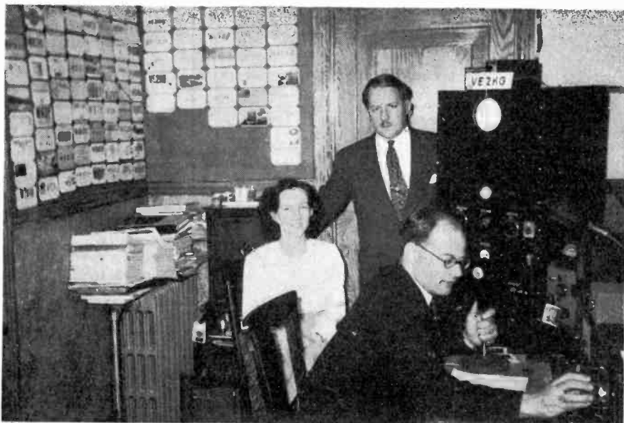
G2CIN, now in Canada, has been visiting many VE's. Here he is (foreground) at VE2KG, Quebec, who has an R.1155 receiver with Emdo converter. The Tx is 6L6-RK39, with 50 watts, into a 4-element beam.
